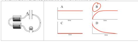
Q19.16b Capacitor initially uncharged. Which graph shows the magnitude of the POTENTIAL DIFFERENCE across the LIGHT BULB FILAMENT while CHARGING?
