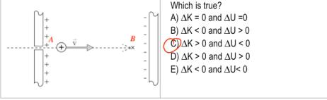
Q16.1b An electron enters a capacitor through a tiny hole. System: everything Which is true?
